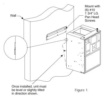
NOTE: If you intend to install this unit with a "WAD" door it must be mounted 1/4" behind front edge of stud.
